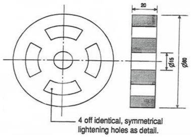
Calculate the volume of the cast iron roller.
