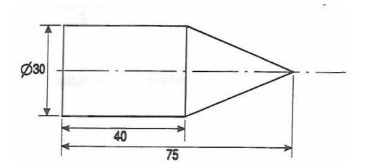
Calculate the volume of the "plumb-bob" shown above. All dimensions are millimetres.
