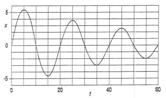
The graph shows that the period of the motion is about 20 seconds. The amplitude starts off at 6 and decays away.
