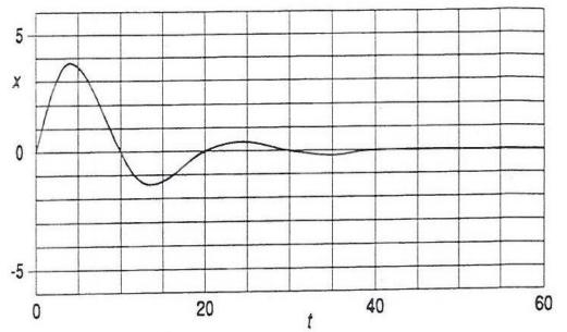
The graph shows that the motion is more heavily damped. The period of the motion is the same. The first maximum, however, occurs well before the 5 second mark.
